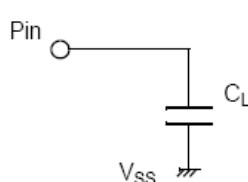
$C_L = 50 \text{ pF}$  (including wiring and probe capacitance).
