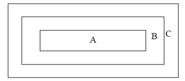
Note: As a general rule, visual defects in Zone C are permissible, when it is no trouble for quality and assembly of customer's product.
