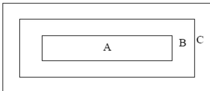
Note: As a general rule, visual defects in Zone C are permissible, when it is no trouble for quality and assembly of customer's product.
