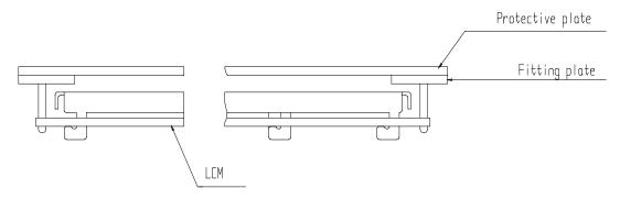
(2) When assembling the LCM into other equipment, the spacer to the bit between the LCM and the fitting plate should have enough height to avoid causing stress to the module surface, refer to the
